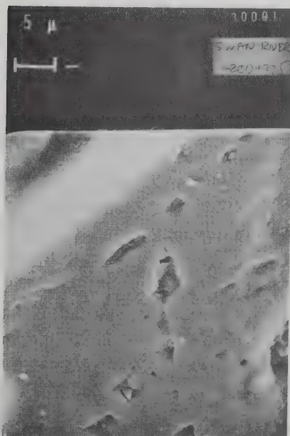
7.5c Swan River Sandstone Solution Pitting. Note lower left to upper right features which control the shape of the pits.
